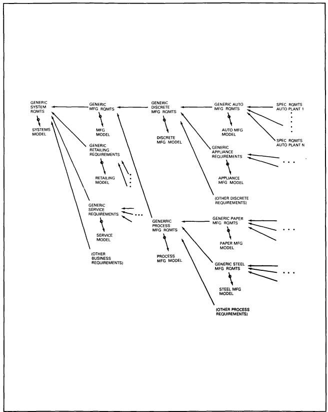
Figure All-I Empirical development of the CIM Reference Model from the requirements of different industries.
